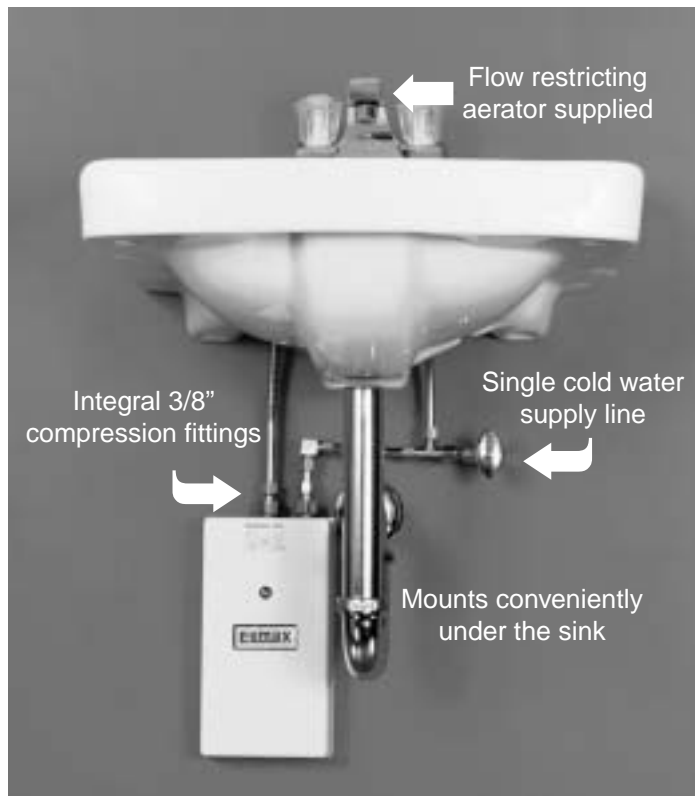
Designed to comply with .5 GPM handwashing code target outlet temperature 105° - 110°.
